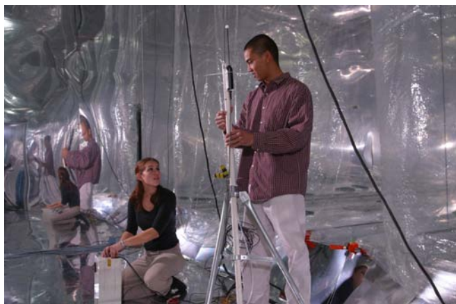
Figure 3. CE-CERT's atmospheric chamber is one of the world's largest indoor facilities where illumination, temperature, and humidity can be controlled.
