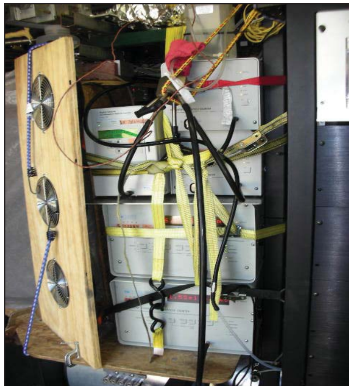
Mounted in the Mobile Emissions Laboratory, this suite of instruments measures particle number in conjunction with a PMP system.
