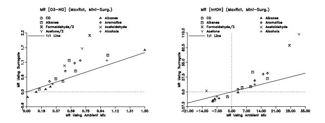
Figure 5. Plots of calculated mechanistic reactivities of selected species in maximum reactivity chamber experiments using the 3-component minisurrogate, against those for similar experiments using the ambient ROG mixture.
