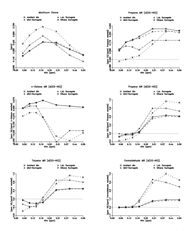
Figure 8. Plots of maximum ozone in base case experiments and of mechanistic reactivities for selected VOCs as a function of initial  $NO_x$  from model simulations of reactivity experiments employing the ambient ROG mixture and selected ROG surrogates.
