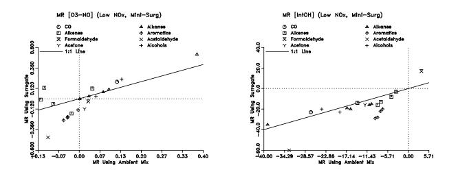
Figure 7. Plots of calculated mechanistic reactivities of representative species in  $NO_x$ -limited chamber experiments using the 3-component mini-surrogate, against calculated mechanistic reactivities for similar experiments using the ambient ROG mixture.
