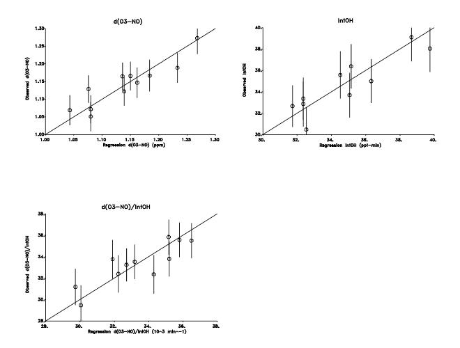
Figure 14. Plots of observed  $\underline{vs}$  regression predicted 6-hour d(O<sub>3</sub>-NO), IntOH and d(O<sub>3</sub>-NO)/IntOH ratios for the base case ethene surrogate experiments.
