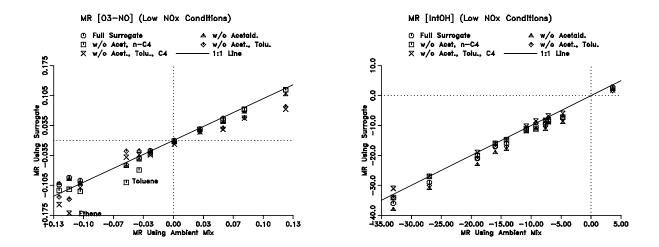
Figure 4. Plots of calculated mechanistic reactivities of selected species in  $NO_x$ -limited chamber experiments using various ROG surrogates, against those for similar experiments using the ambient ROG mixture.
